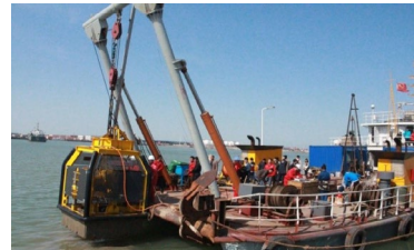
Demonstration of offshore cone penetration test
